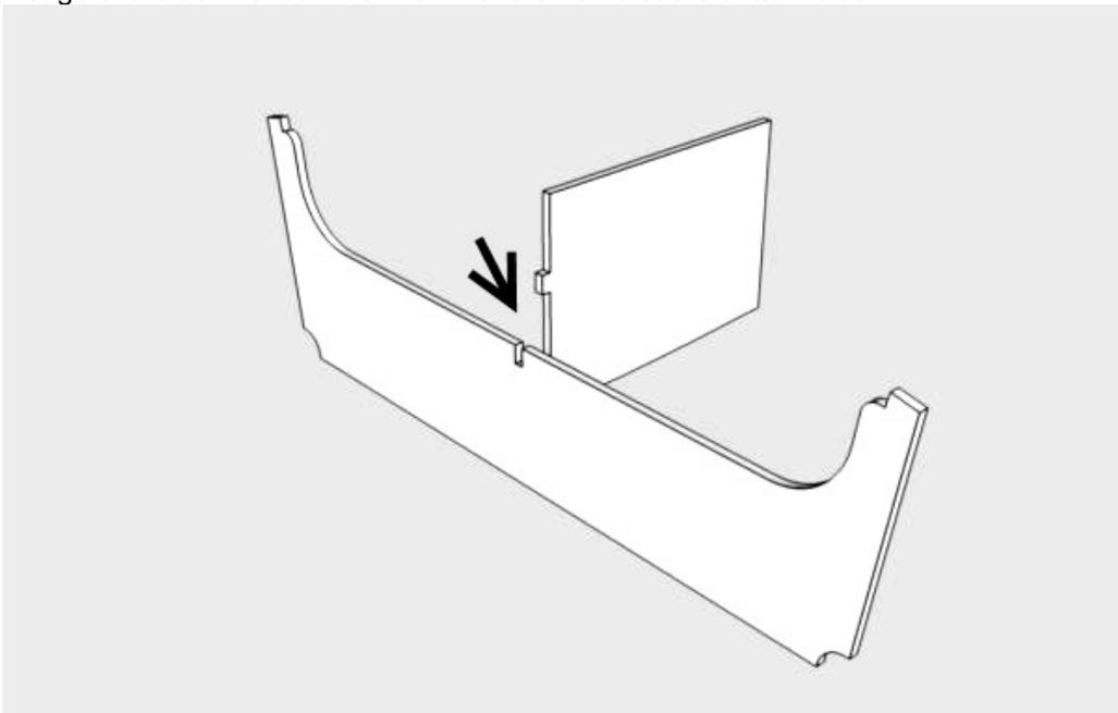
Once you are satisfied with the way the tab fits in the notch, disassemble the parts and put them aside.
