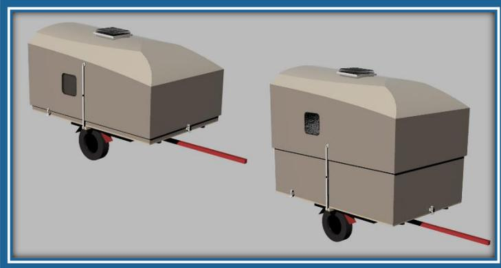
This trailer collapses vertically. Common teardrop type trailers have limited headroom. So, you crawl inside and you're sitting on the bed. With minimal extra complexity, this trailer raises up 24" / 610mm (with gas springs to help) and gives standing headroom at the back end. It's much roomier inside, but when it's time to trailer, the lower profile gives a very good aerodynamic shape. It's much better than the flat or blunt profiles of some small teardrop trailers.
