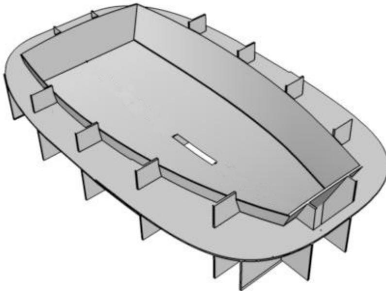
Still no fasteners. Note the cut for the dagger board trunk in the sole. The sole panel is supplied with a
