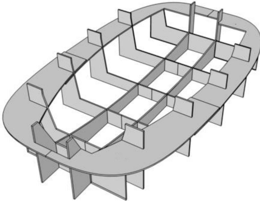
The sturdy basket mold is made from Fir marine plywood 3/4" thick. All parts are notched for easy assembly. The mold goes together like a puzzle, there is nothing to measure. The mold should be installed on a stable flat surface: floor, low table or some 2x4's on saw horses.
