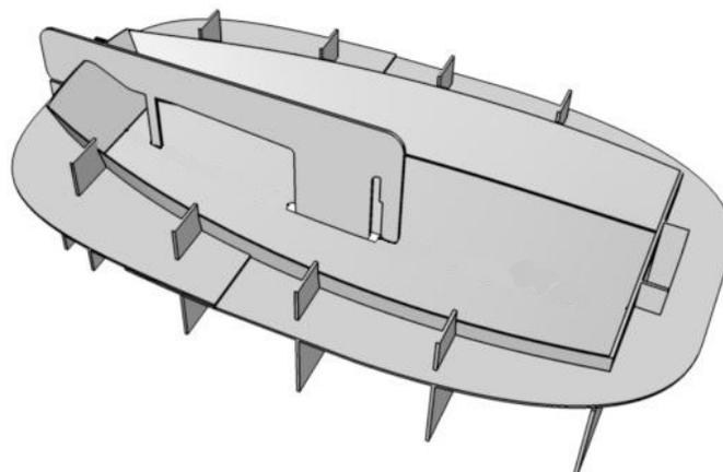
The locator extends through the slot in the bottom and is marked at the front to line up with the bow transom.
