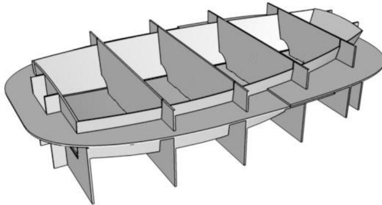
The inside frames have openings at the chine to allow the builder to install fiberglass tape in one piece.
